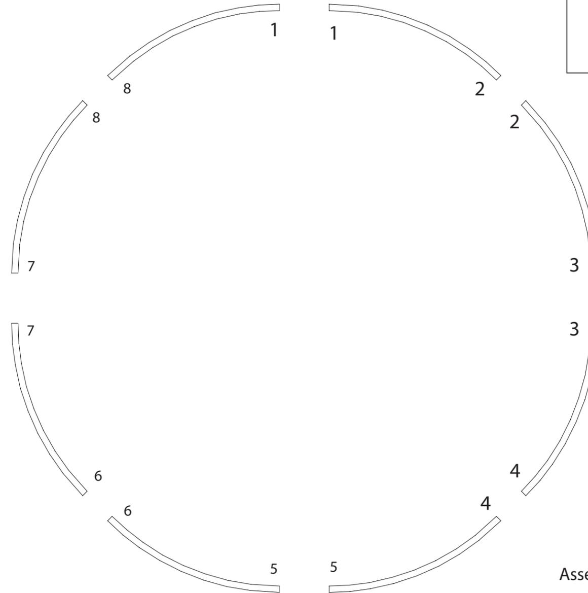
Assemble aero frame parts in numerical order.
